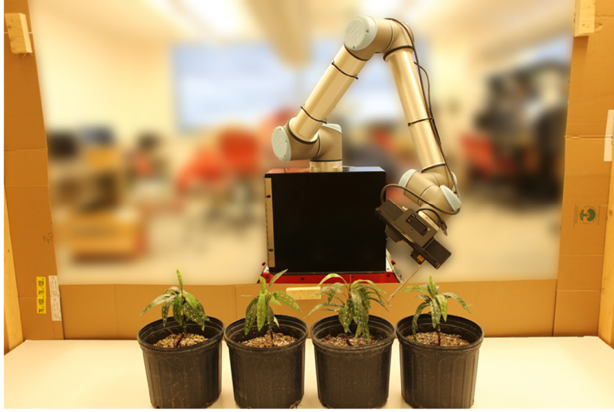
Figure 1. Robotic leaf probing of artificial plants in a growth chamber mock-up. The system includes a six-axis UR10 robotic manipulator, a Kinect V2 sensor, a Keyence LJ-V7300 2D in-line laser profilometer, and a probe.
